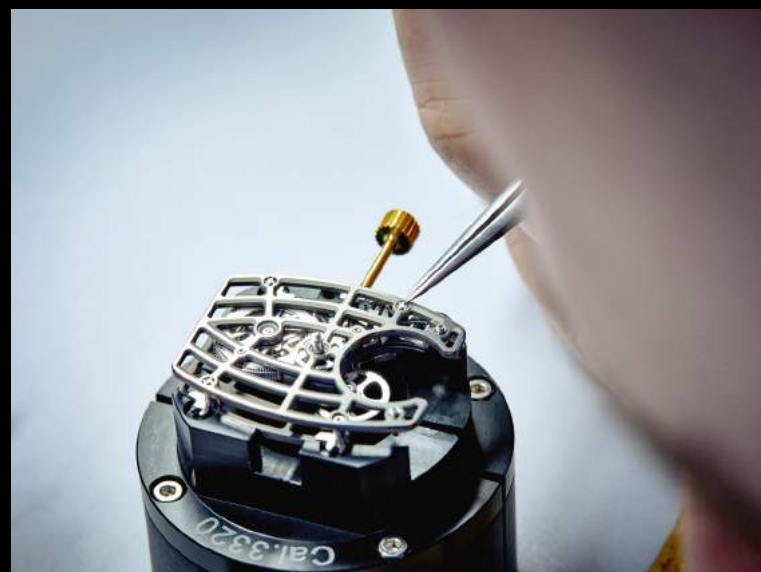
Careful tightening of the spline screws that secure the upper bridge of the RM 71-01
