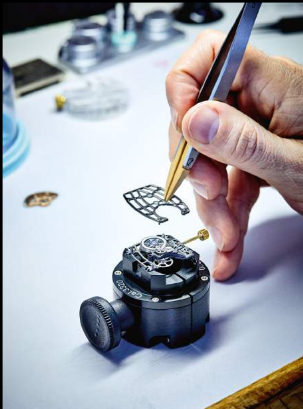
Incorporation of the upper bridge made of grade 5 titanium
