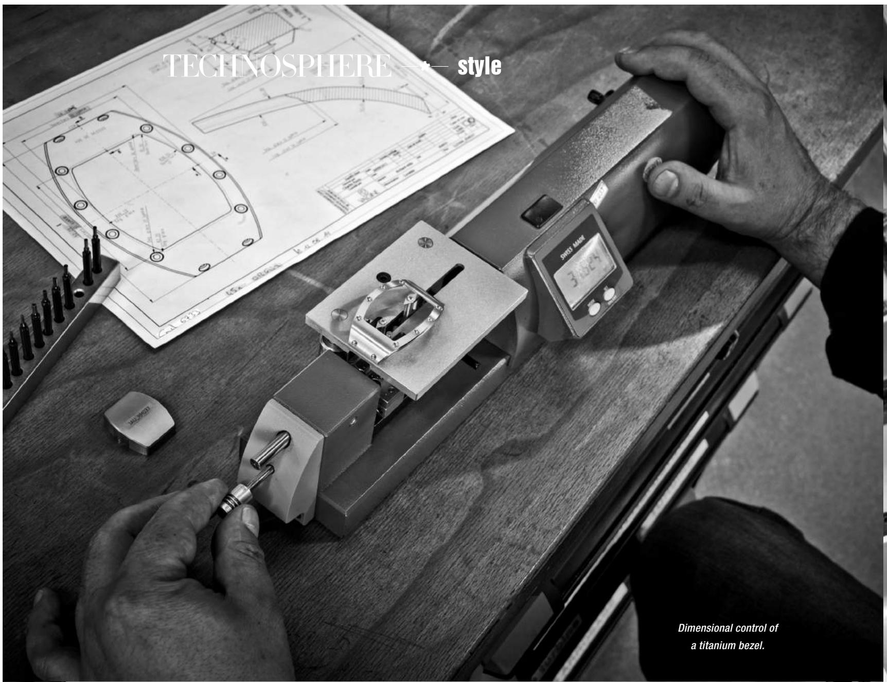
*Dimensional control of a titanium bezel.*
