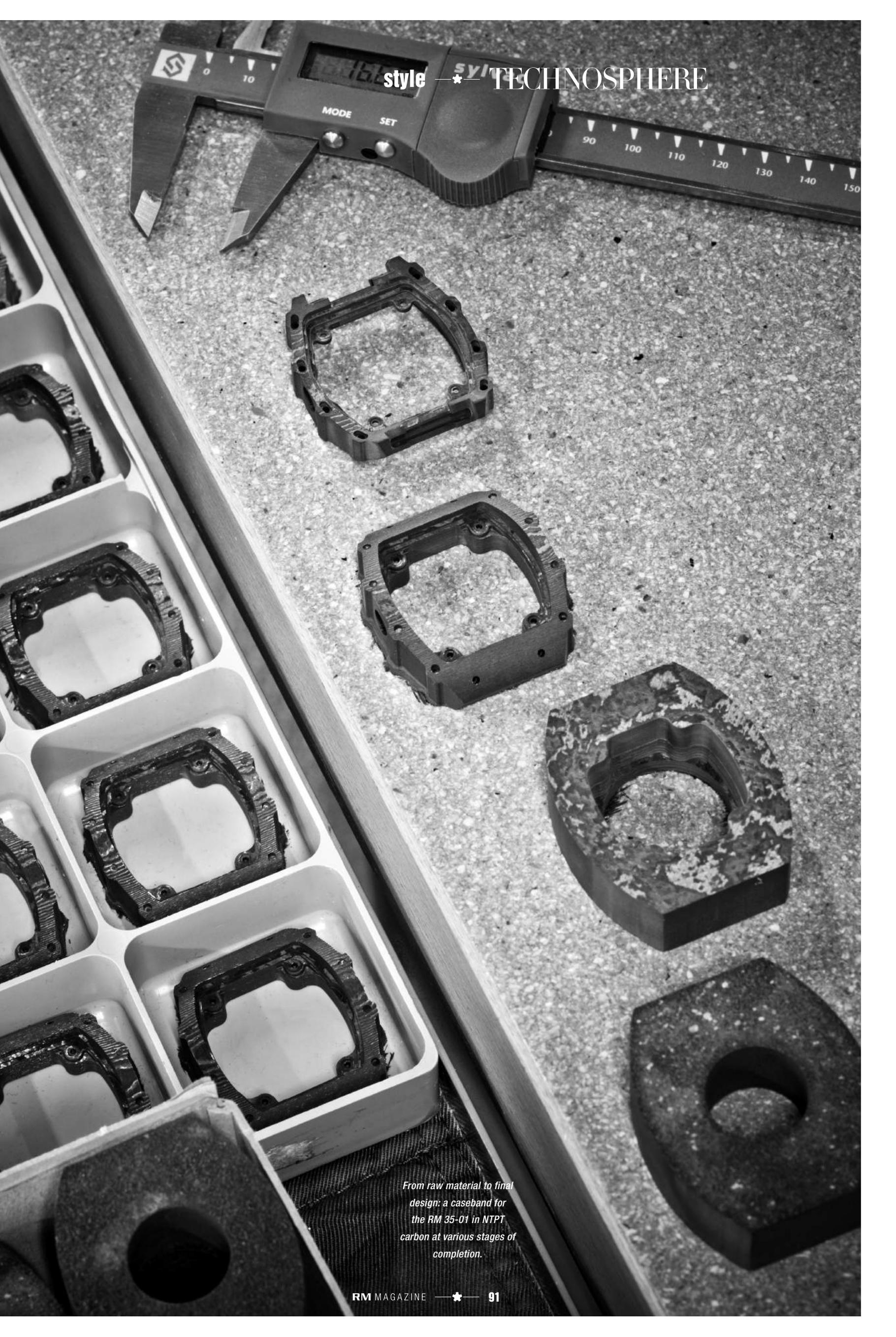
*From raw material to final design: a caseband for the RM 35-01 in NTPT carbon at various stages of completion.*
