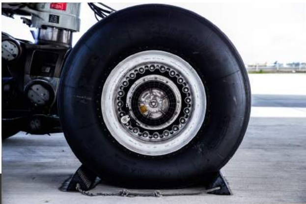
Special Michelin tyres on the A350-900 are lighter and resistant to damage, reducing unscheduled maintenance
